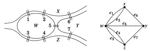
The model on the right makes it easy to argue that the desired traversal does not exist. Each time we enter and leave a land mass, we use two bridges ending at it. We can also pair the first bridge with the last bridge on the land mass where we begin and end. Thus existence of the desired traversal requires that each land mass be involved in an even number of bridges. This necessary condition did not hold in Königsberg.
