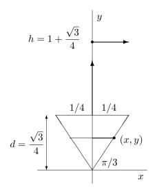
To calculate the vertical depth of the tank you can use the Pythagorean Theorem:
