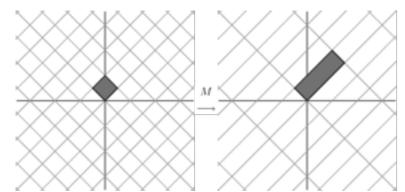
Ah ha. We see now that this new grid is transformed in the same way that the original grid was transformed by the diagonal matrix: the grid is stretched by a factor of 3 in one direction.
