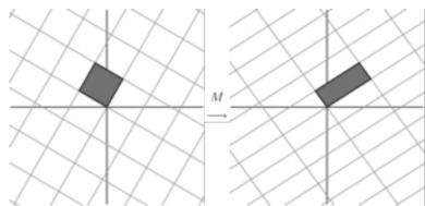
Hmm. It appears that the grid on the right is now almost orthogonal. In fact, by rotating the grid in the domain by an angle of roughly 58.28 degrees, both grids are now orthogonal.
