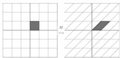
It's easy to find one family of eigenvectors along the horizontal axis. However, our figure above shows that these eigenvectors cannot be used to create an orthogonal grid that is transformed into another orthogonal grid. Nonetheless, let's see what happens when we rotate the grid first by 30 degrees,
