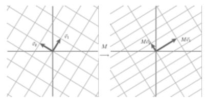
We will use  $\mathbf{u_1}$  and  $\mathbf{u_2}$  to denote unit vectors in the direction of  $M\mathbf{v_1}$  and  $M\mathbf{v_2}$ . The lengths of  $M\mathbf{v_1}$  and  $M\mathbf{v_2}$ -denoted by  $\sigma_1$  and  $\sigma_2$ -describe the amount that the grid is stretched in those particular directions. These numbers are called the *singular values* of M. (In this case, the singular values are the golden ratio and its reciprocal, but that is not so important here.)
